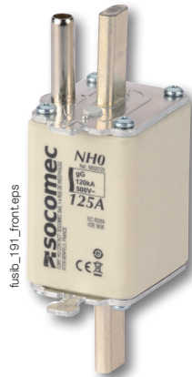
gG type fuse, NH0, with striker from 16 to 200 A
